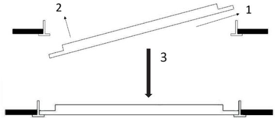
Adjust the module position to fit ceiling well.
