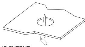
**CEILING CUTOUT:** 25W = Ø165-180 mm $13W = \emptyset 95-100 \text{ mm}$
