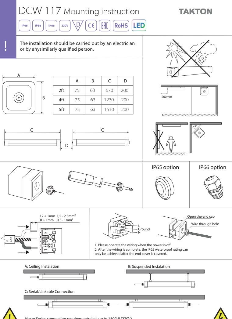
Macro Series connection requirements: link up to 1800W (220V) cable length is within 100 meters
